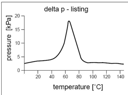
During ramp measurements, with every ignition a small amount of vapor is being burned. Typically this effect is negligible or can be controlled. For example if the ignition is not being set every 1°C, but for example every 3°C. This allows more vapors to be formed, before the next ignition is being set.
