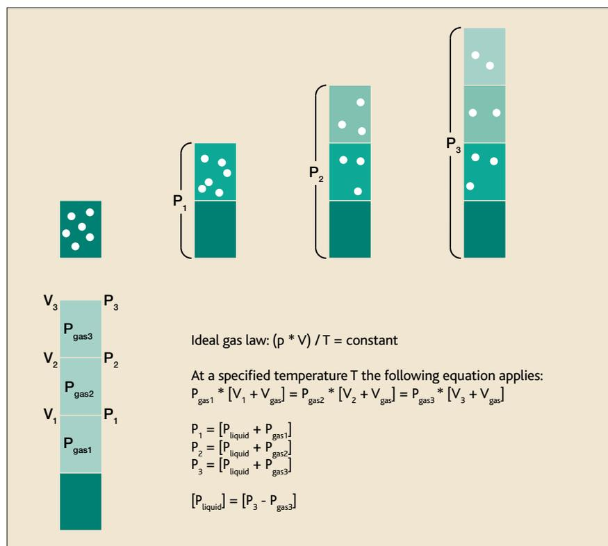
Figure 2 Vapour pressure measurement using the triple expansion method
